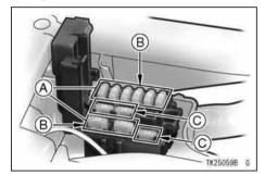
A. Fuse Box B. Fuses C. Spare Parts
