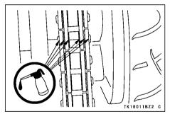
• If the chain is especially dirty, clean it using diesel oil or kerosine and then apply oil as mentioned above.
