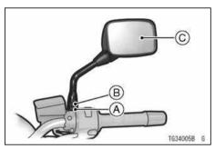
A. Lower Hexagonal Area for Tightening
