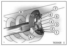
A. Spring Preload Adjuster B. Wrench
