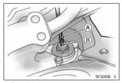
A Screwdriver B. Rebound Damping Force Adjuster
